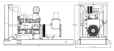
Drawing above for illustration purposes only, based on standard open power 480 volt engine-generator set. Lengths may vary with other voltages. Do not use for installation design. See website for unit specific template drawings.
